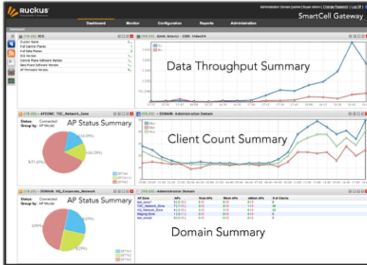
Inspired by real-world experience with carriers operating some of the world's largest Wi-Fi networks, the SCG's element management system provides a wealth of detailed controls, statistics, reporting, and troubleshooting tools, along with northbound interface options for integration into carrier network management systems.
