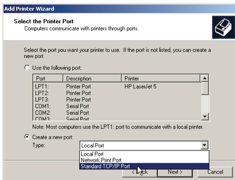
5. The Add Standard TCP/IP Printer Port Wizard box will then appear as shown the pictures below, and type in the IP address assigned to the print server in the **Printer Name or IP Address** box, Click **Next**.
