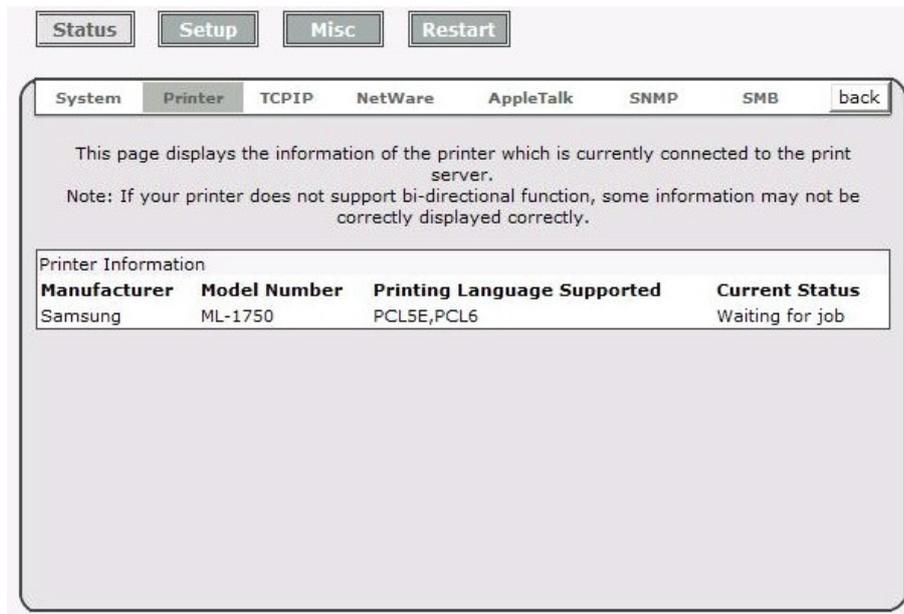
**Manufacturer:** This option allows you to view manufacturer of the printer. When the printer connected with the print server, it will be show in the manufacture box.
