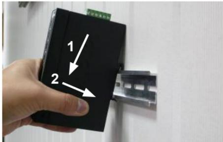
**Step 3:** Check the DIN-Rail is tightly on the track.
