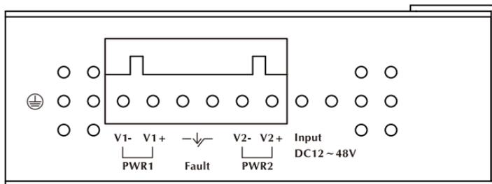
**Figure 2-6** Industrial Fast Ethernet Switch upper Panel.
