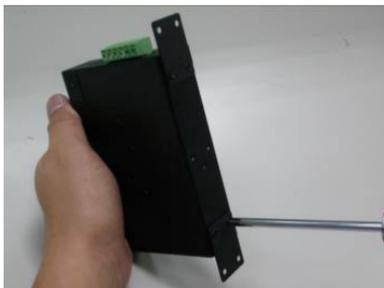
**Step 3:** Use the screws to screw the wall mount plate on the Industrial Fast Ethernet Switch.
