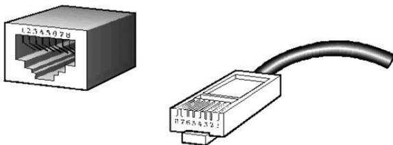
The standard RJ-45 receptacle/connector
