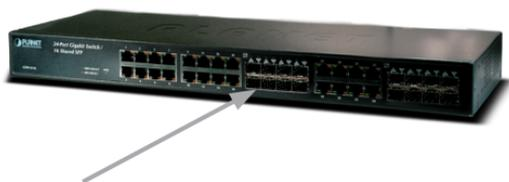
**Figure A-2** Insert the Mini-GBIC modules
