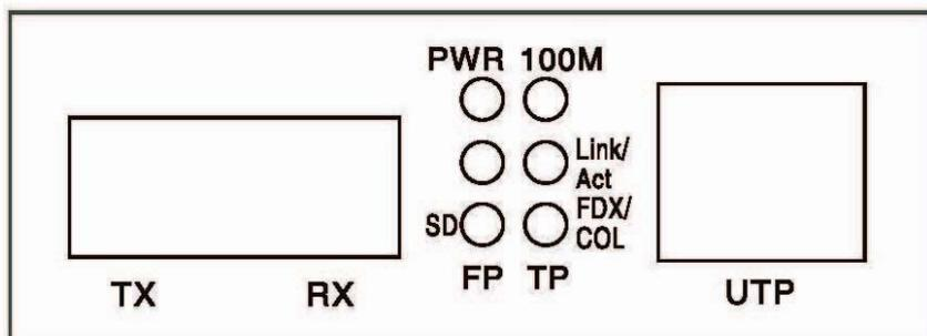
Fig. 2 Converter Front Panel for external power
