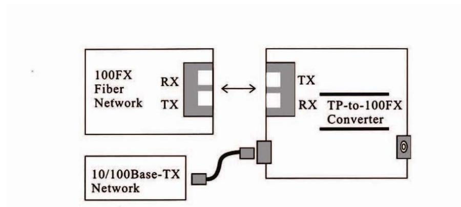
Fig. 1 Basic Network Connection
