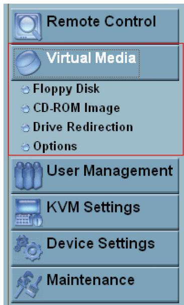
Drive Redirection allows you to share (redirect) your local drive (floppy drives, hard disks, CD ROMs and other removable devices like USB sticks) with the remote system over a TCP network connection. Thus, with Drive Redirection, you can use a virtual disk drive on the remote computer instead of an image file. It is also possible to enable a remote machine to write data to your local disc.
