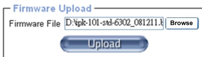
In order to do that you need to select the file on your local system using the button "**Browse**" of the Upload Firmware panel. Click **Upload**. Once the firmware file has been uploaded, it is checked whether it is a valid firmware file and whether there were any transmission errors. In case of any error the Upload Firmware function will be aborted.
