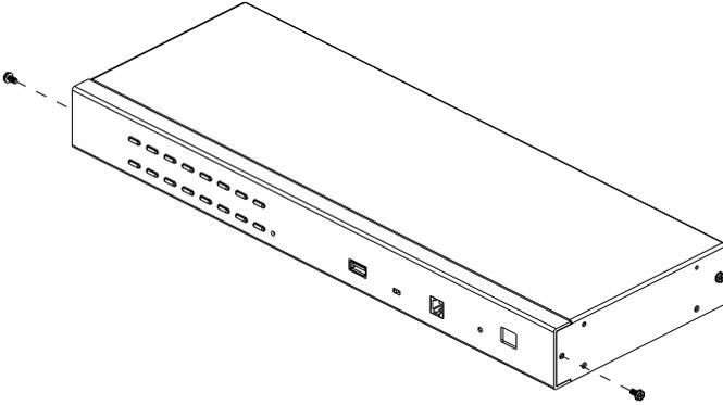
2. Use the M3 x 8 Phillips hex head screws supplied with the rack mounting kit to screw the rack mounting brackets into the sides near the front of the unit.
