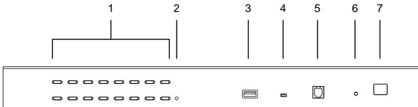
**Note:** The CS1716A is pictured above. The CS1708A front panel is the same as the CS1716A, except that it has 8 KVM port LEDs instead of 16.
