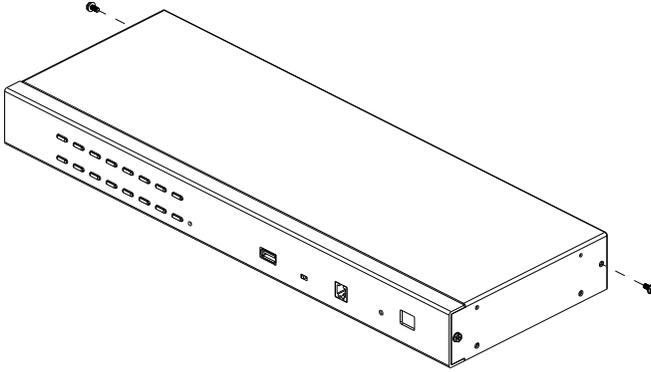
2. Use the M3 x 8 Phillips hex head screws supplied with the rack mounting kit to screw the rack mounting brackets into the sides near the rear of the unit.
