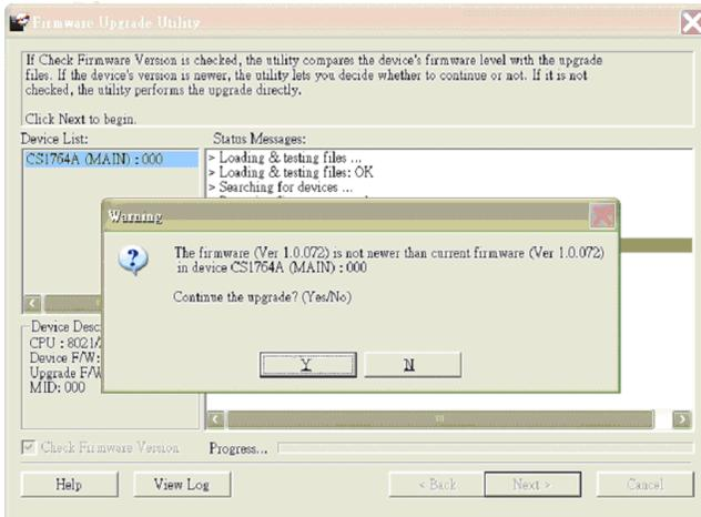
If you didn't enable *Check Firmware Version*, the Utility installs the upgrade files without checking whether they are a higher level, or not.
