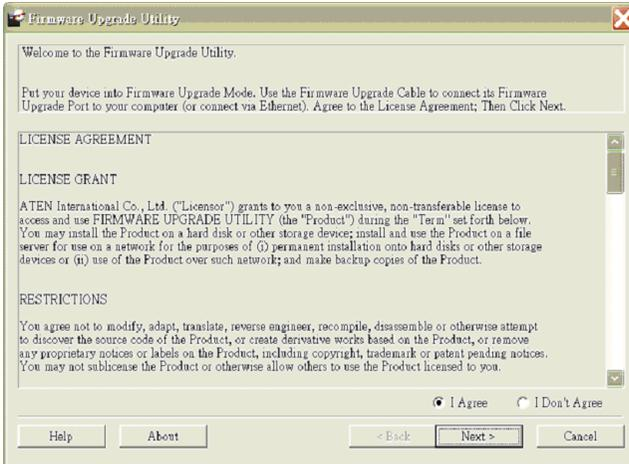
3. Click **Next**. The Firmware Upgrade Utility main screen appears. The Utility inspects your installation. All the devices capable of being upgraded by the package are listed in the *Device List* panel.
