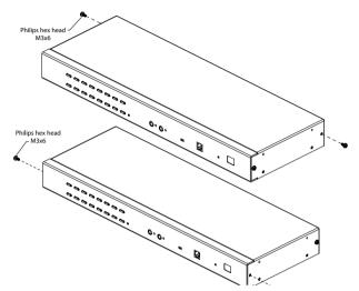
2. Screw the mounting brackets into the sides of the unit at the front or the rear, as shown in the diagram below.
