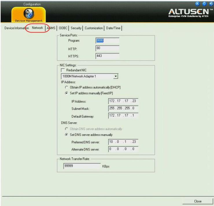
The screenshot shows the ALTUSCN Configuration window with the 'Network' tab selected. The 'Network' tab is circled in red. The window displays the following settings:
