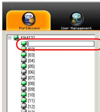
2. Key in a name for the port (or change/delete a previous one). The maximum number of characters allowed for a port name is 20. You can use any combination of letters, numbers, and symbols on the typewriter keys of keyboards with PC US English layout.
