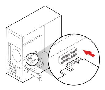
Step 3: Connect the other end of the Bluetooth® cable to the motherboard F\_USB (front USB) 9-pin header. Ensure correct keying—incorrect insertion will cause Bluetooth to malfunction.
