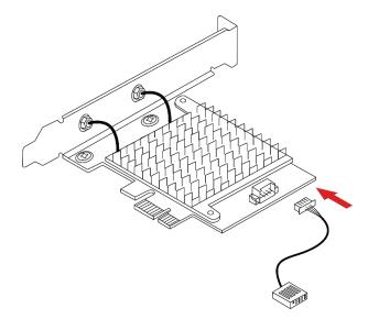
Step 2: Insert the Bluetooth® interface cable into the USB header on the accessory end of the network card. Pay attention to the pin-1 orientation.
