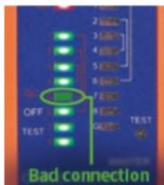
If the connector is not connected properly to the wire-harness, the indicator light of the wire harness will not be turned on.
