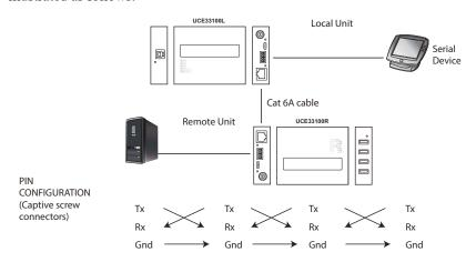
The general concept here is that a RS-232 signal can be transmitted (Tx) to the receiving (Rx) end of a unit. The received signal can then be transmitted (Tx) to the receiving (Rx) end of another unit. The RS-232 signals can be transmitted back the other way.
