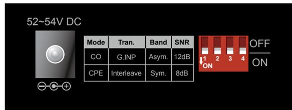
For point-to-point connection, the VC-231GP in the CPE mode and the VC-231G or VC-234G in the CO mode must be set up as one pair of converters to perform the connection. It gives administrators the ability to reply a fresh local Intranet in various locations by utilizing the original network structure without additional costs.
