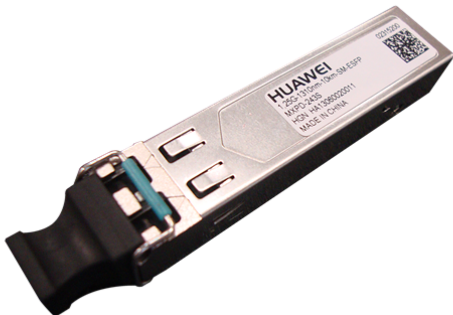
Figure 10-3 SFP/eSFP optical module
