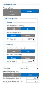
On Stop periodic tracking - enable or disable periodic data sending when device is On Stop. Device will generate and send normal record with event ID 0 and movement AVL ID 240 with a value of 0.
