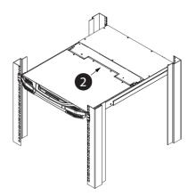
3. While one person hold the weight of the LCD KVM switch, have a second person install four screws in the front tabs to secure the module to the front of the rack.
