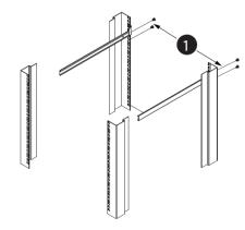
2. Two people insert the LCD KVM switch, by sliding its left and right side bars into the mounting brackets.
