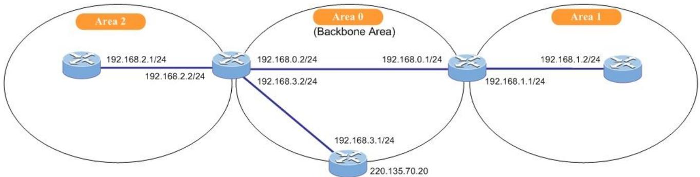
Following is OSPF area configuration table. It is used to specify the OSPF enabled interface(s). When OSPF is enabled on the specific interface(s), the router can provide the network information to the other OSPF routers via those interfaces. The screen in [Figure 4-10-4-2](#) appears.
