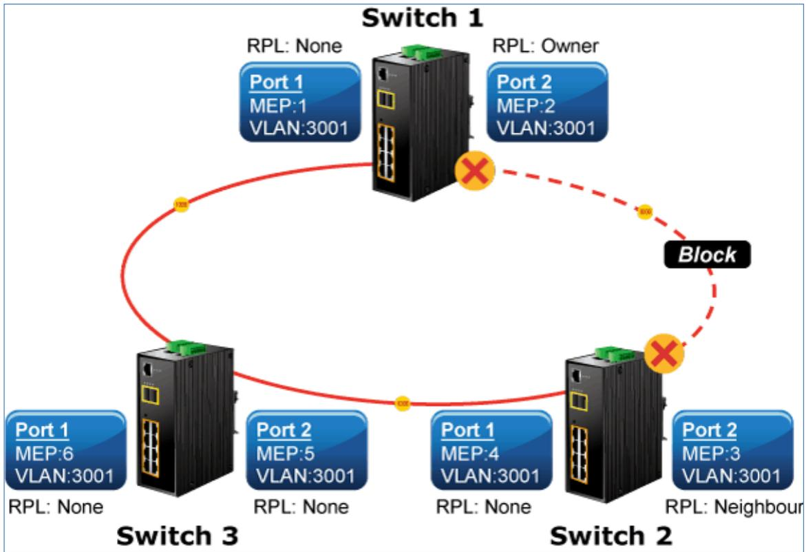
Figure 4-6-4-2: Ring Example Diagram
