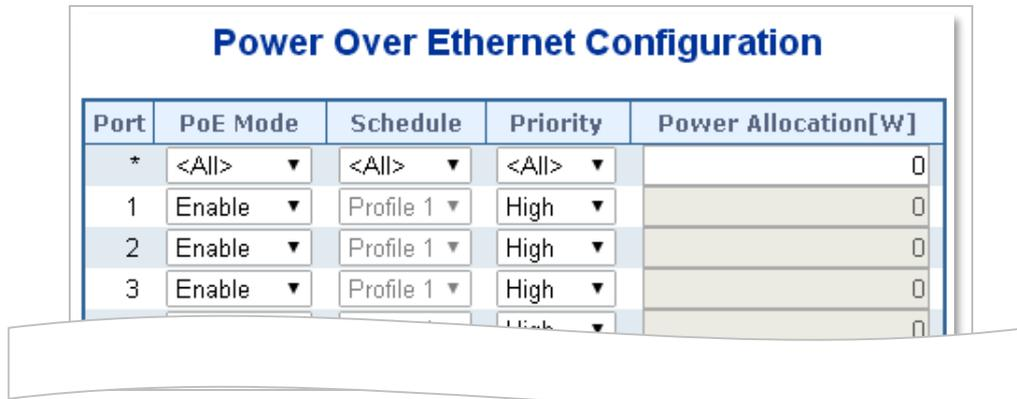
**Figure 4-8-4-1:** Power over Ethernet Configuration Screenshot
