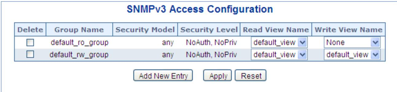
The screenshot shows the 'SNMPv3 Access Configuration' interface. It features a table with the following columns: Delete, Group Name, Security Model, Security Level, Read View Name, and Write View Name. There are two entries in the table: 'default\_ro\_group' and 'default\_rw\_group'. Below the table are three buttons: 'Add New Entry', 'Apply', and 'Reset'.
