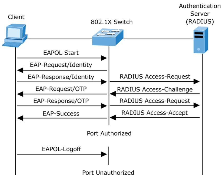
Figure 4-5-2-2: EAP Message Exchange
