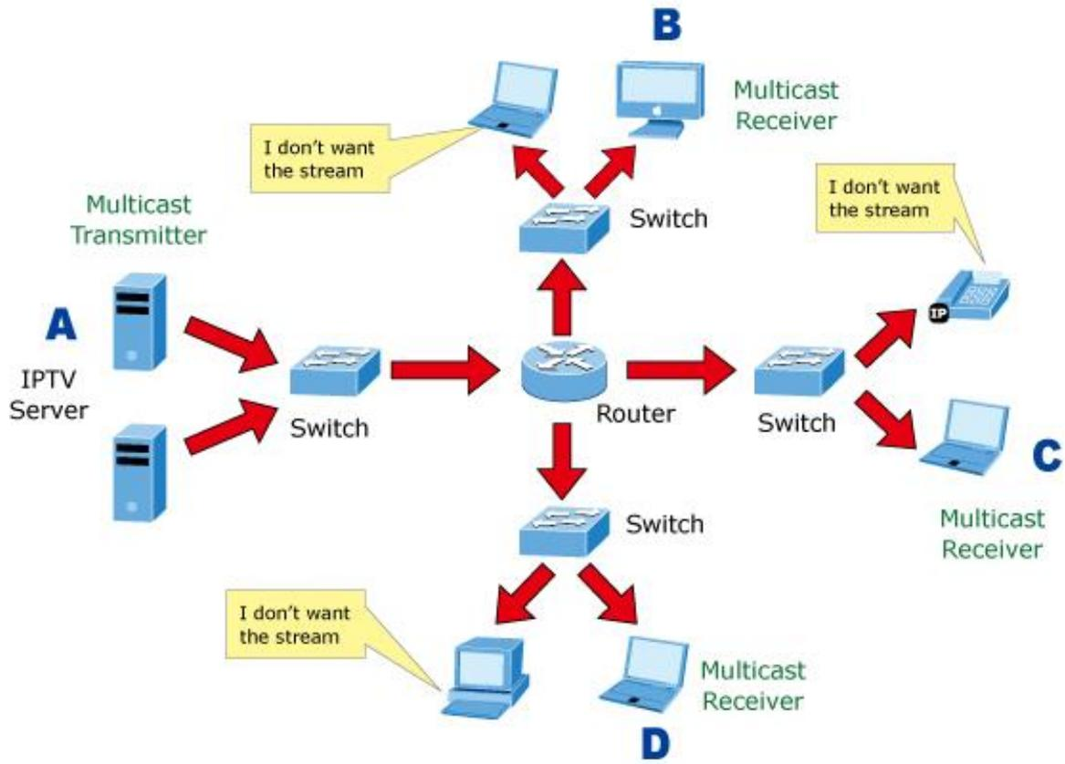
Figure 4-3-9-2: Multicast Flooding
