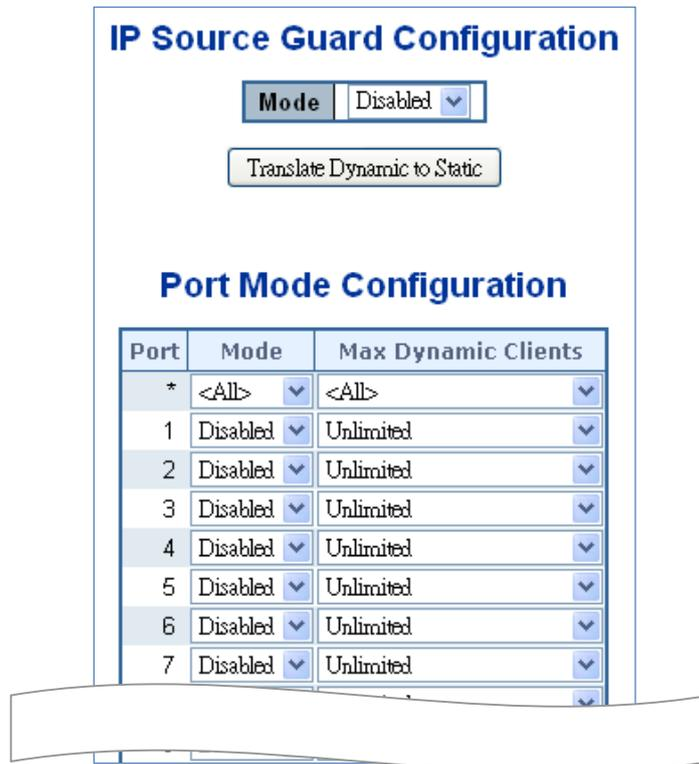
Figure 4-5-7-1: IP Source Guard Configuration Screen Page Screenshot
