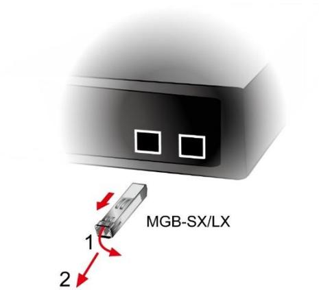
**Figure 2-2-5:** How to Pull Out the SFP Transceiver
