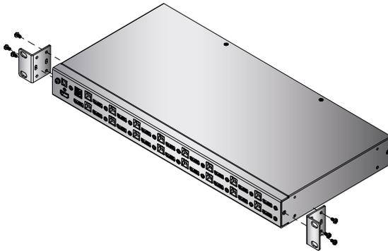
3. Place the KVM switch in the rack. Position it so that the holes in the mounting brackets line up with the holes in the rack. Secure the mounting brackets to the rear of the rack.
