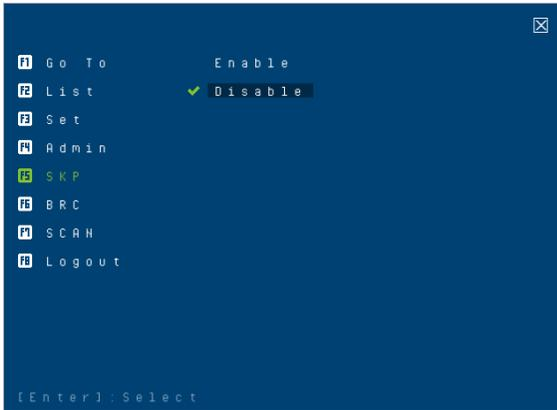
Clicking **F5 SKP** or pressing **F5** invokes Skip (SKP) mode. This function enables you to easily skip backward or forward – switching the console focus from the currently active computer port to the previous or next accessible one. Enable mouse emulation for Skip mode to work (see page 41).
