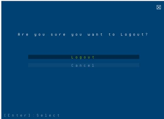
Clicking **F8** **L o g o u t**, or pressing **F8** logs you out of OSD control of the computers, and blanks the console screen. This is different from simply pressing **Esc** when you are at the main screen to deactivate the OSD. With this function you must log in all over again to regain access to the OSD, whereas with **Esc**, all you have to do to reenter the OSD is tap the OSD hotkey.
