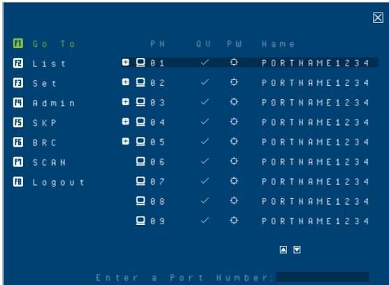
Clicking **F1 G O T O** or pressing **[F1]** activates the Go To function. Go To allows you to switch directly to a port by keying in the port's ID. Enable mouse emulation for independent switching (see page 41), for this function to work.
