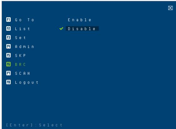
F6 is an administrator only function. Clicking **F6 BRC** or pressing **[F6]**, invokes *Broadcast* (BRC) mode. When this function is in effect, commands sent from the console are broadcast to all available computers on the installation.
