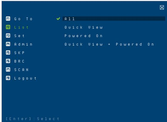
Clicking **F2 List** or pressing **[F2]** activates the List function. This function lets you broaden or narrow the scope of which ports the OSD displays on the main screen. The submenu choices and their meanings are given in the table below.
