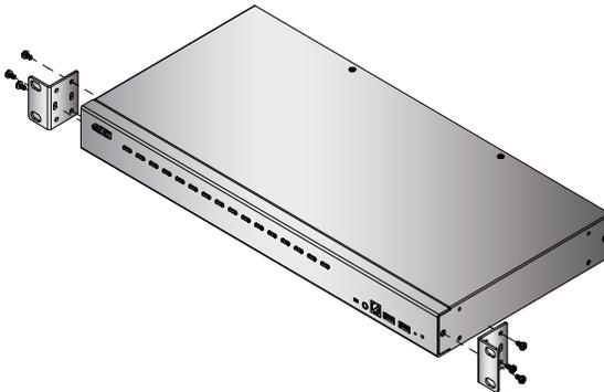
3. Place the KVM switch in the rack. Position it so that the holes in the mounting brackets line up with the holes in the rack. Secure the mounting brackets to the front of the rack.
