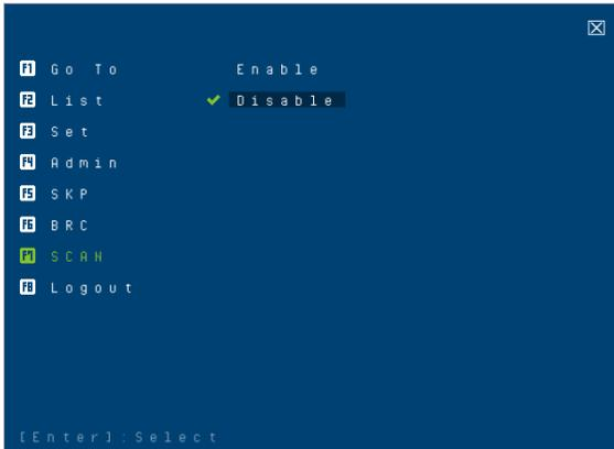
Clicking **F7** **SCAN** or pressing **[F7]** invokes *Auto Scan* mode. This function allows you to automatically switch among the available computers at regular intervals so that you can monitor their activity without having to take the trouble of switching yourself. Enable mouse emulation for *Auto Scan* to work (see page 41).
