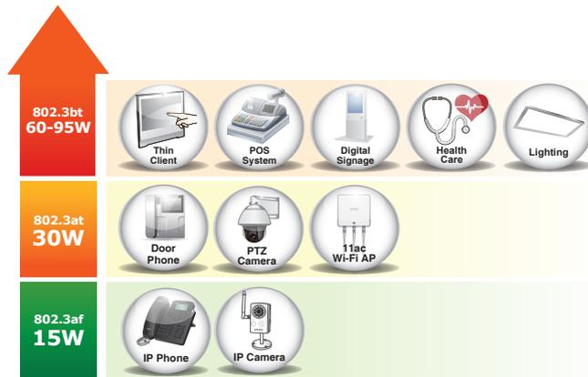
**Built-in Unique PoE Functions for Powered Devices Management**
