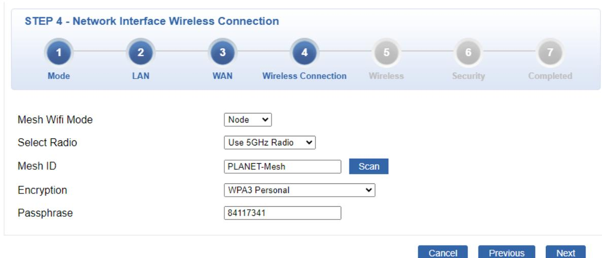
Figure 4-12: Wireless Connection-MESH set up
