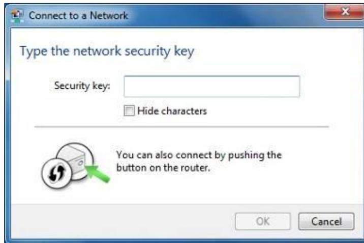
**Figure 5-6** Typing the Network Key
