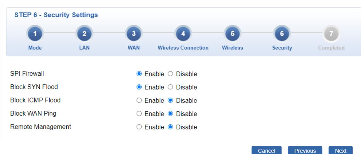
**Figure 4-14:** Setup Wizard –Security Setting
