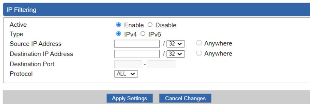
**Figure 4-45: IP Filter Rule Setting**
