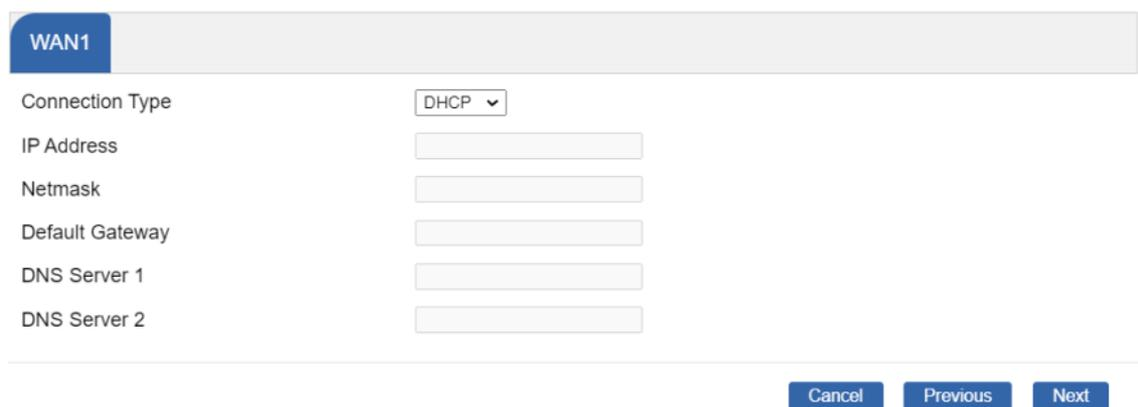
The screenshot shows the WAN1 configuration interface. At the top, there is a tab labeled 'WAN1'. Below it, the 'Connection Type' is set to 'DHCP' in a dropdown menu. There are six input fields for 'IP Address', 'Netmask', 'Default Gateway', 'DNS Server 1', and 'DNS Server 2', all of which are currently empty. At the bottom right of the interface, there are three buttons: 'Cancel', 'Previous', and 'Next'.
