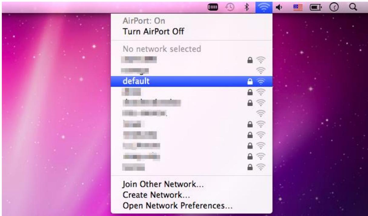
**Figure 5-10** Highlighting and Selecting the Wireless Network
