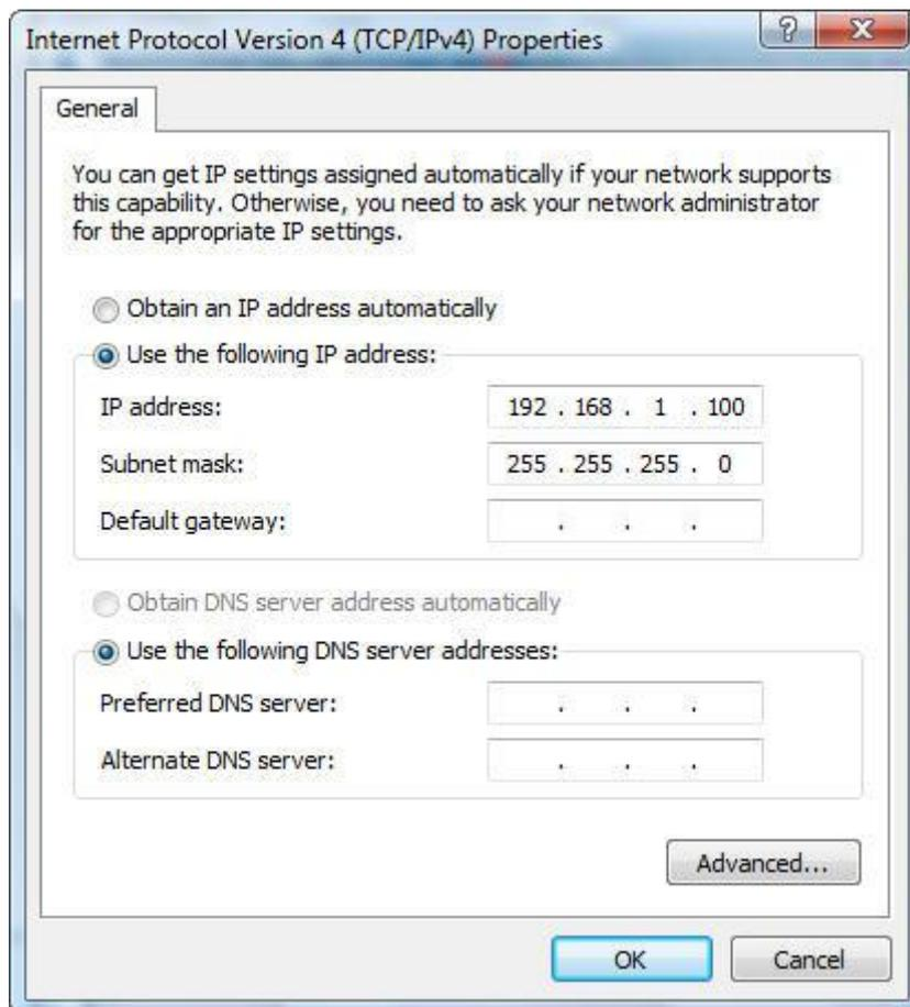
Figure 3-6 TCP/IP Setting
