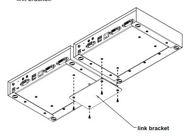
2. Remove the bottom and side screws from each KE Series unit.
