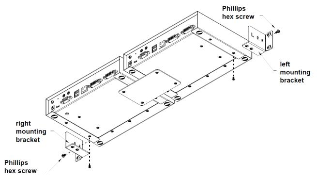
4. Screw the mounting brackets to the rack.
