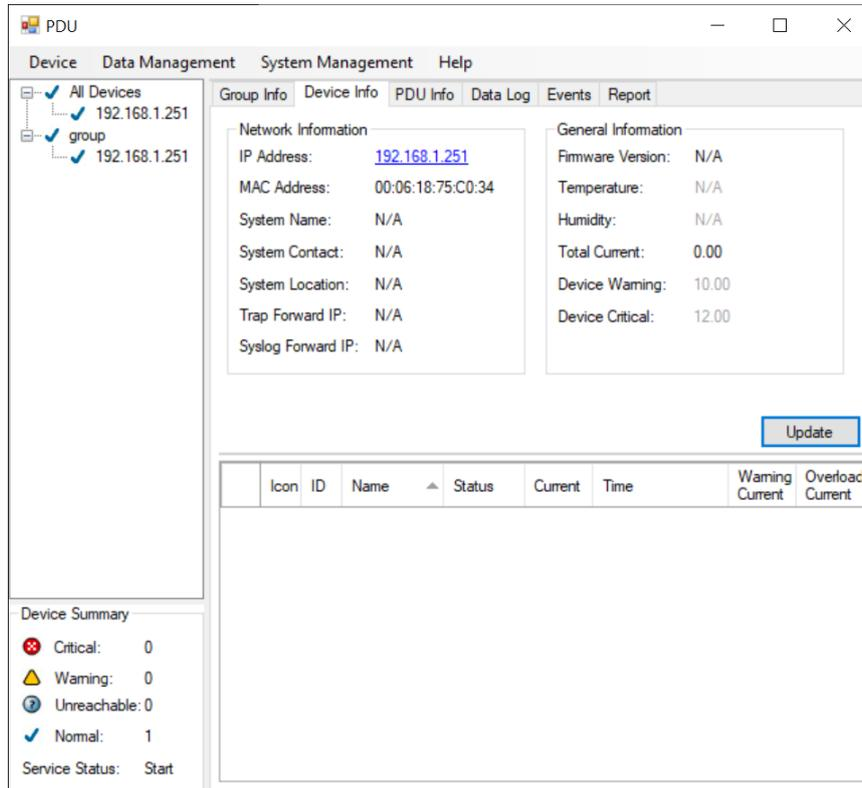
Indicates all relevant information for the connected PDU.
