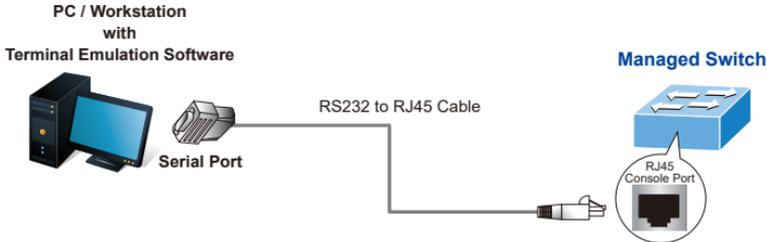
Figure 4-1 Managed Switch Console Connectivity
