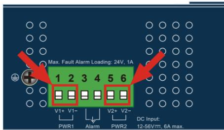
2. Tighten the wire-clamp screws for preventing the wires from loosening.
