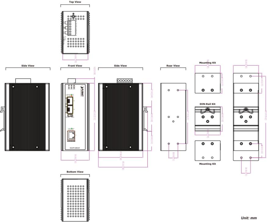
Figure 1: IGUP-1205AT Three-View Diagram
