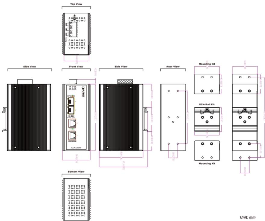
Figure 2: IGUP-2205AT Three-View Diagram
