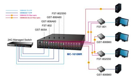
The MC-1610MR series is designed with hot-swappable slot and provides redundant link function to avoid the shutdown of the entire network. PLANET Managed Media Converter Chassis with FST-80x/GST-80x series Fast/Gigabit Ethernet Smart Media Converters are an ideal solution to building a reliable FTTC (Fiber to the Curb) or FTTB (Fiber to the Building) network solution for ISPs, campuses and enterprises.
