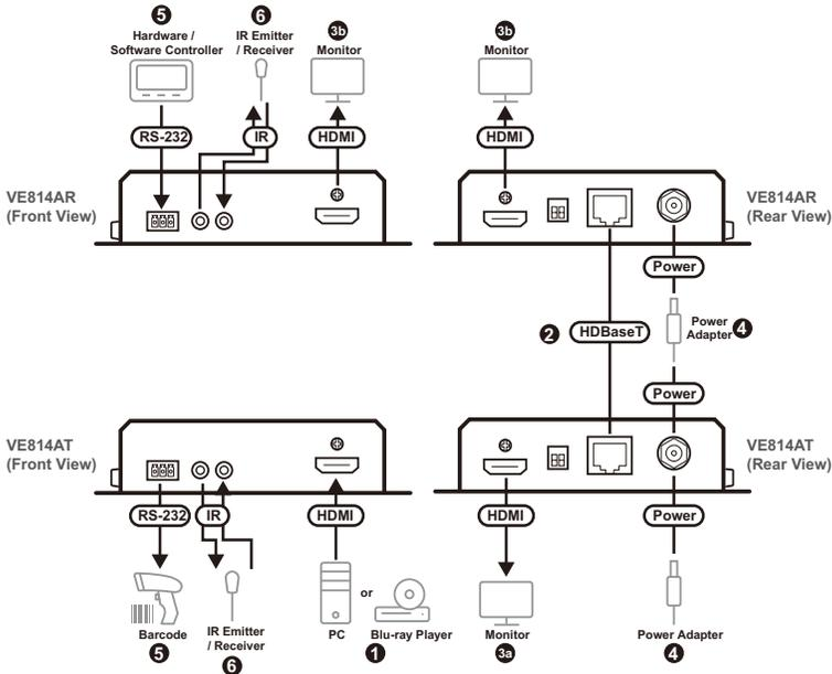
1. Connect the HDMI in port on the VE814AT to the HDMI out port on your video source device using an HDMI cable.
