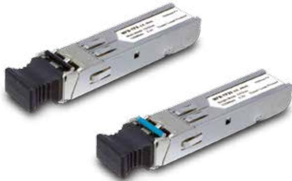
The MFB family consists of Small Form Factor Pluggable (SFP) transceiver modules that are specifically designed for high performance integrated duplex data link over single mode optical fiber. These transceiver modules are compliant with the SFP Multisource Agreement (MSA) and hot pluggable. These modules offer an easy way to be installed in SFP MSA compliant ports at any time without the interruption of the host equipment operation.
