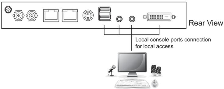
This access is similar to using the server/computer directly. The CN9000/CN9600/CN9950 is able to split the signal to both the local and remote consoles.
