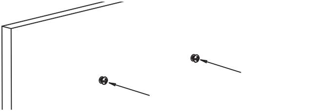
2. Hang the unit to the hanging hooks matching the bracket's hanger keyholes.
