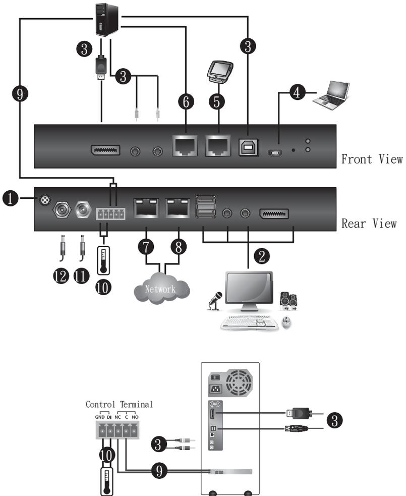
**Note:** When the input device's monitoring parameter (e.g. temperature or humidity) exceeds the set threshold, 1 is sent to the unit, otherwise, 0 is sent.
