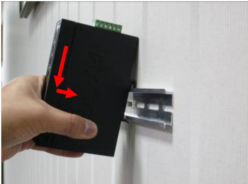
**Step 2:** Check whether the DIN-rail is tightly on the track.
