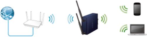
In this mode, the user can access wireless AP, devices can be connected to other wireless network using the wireless, all interfaces are bridging together. Without NAT, firewall and all network related functions.
