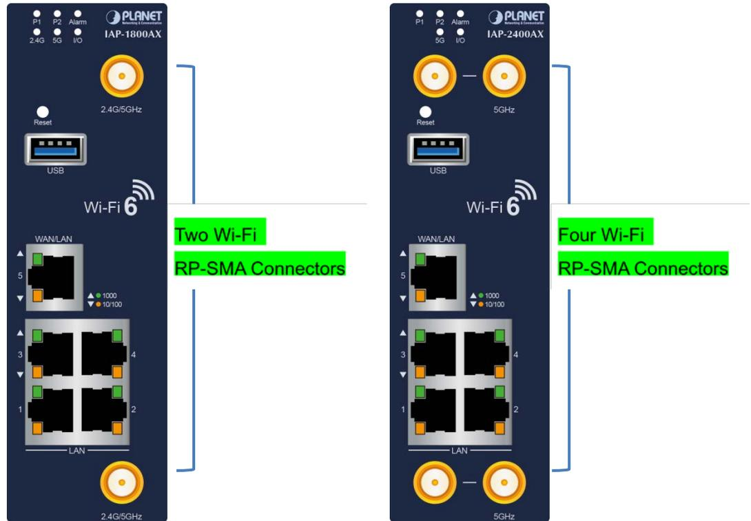
**Figure 2-2:** Industrial 802.11ax Wireless AP Front Panels
