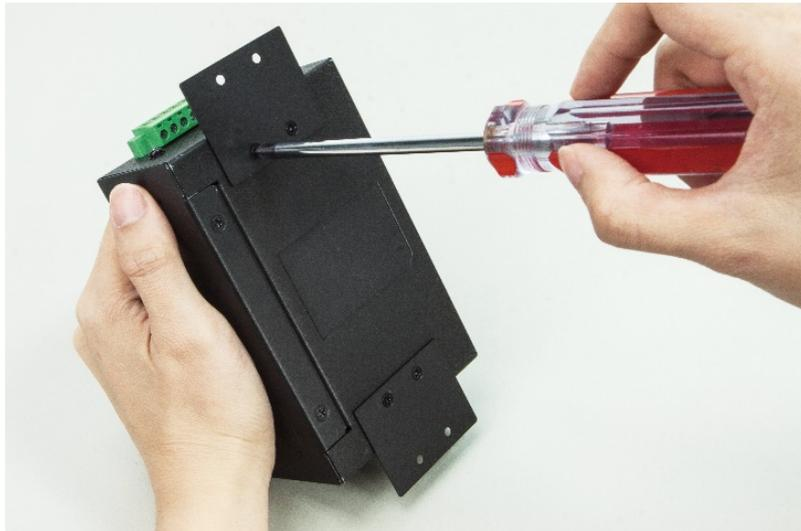
**Step 3:** Use the hook holes at the corners of the wall mount plate to hang the Industrial 802.11ax Wireless AP on the wall.
