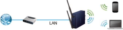
In this mode, the AP wireless interface and cable interface are bridging together. Without NAT, firewall and all network related functions.
