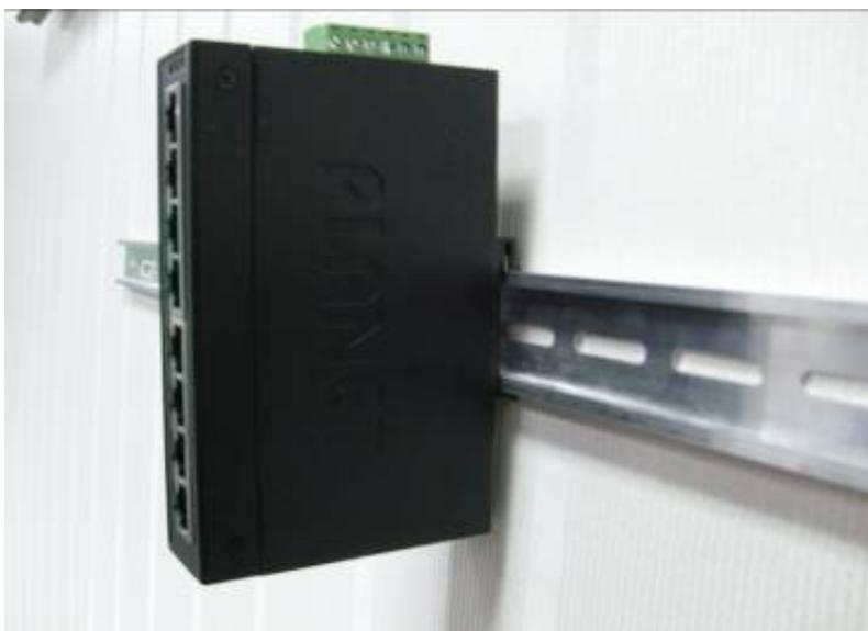
**Step 3:** Lightly remove the DIN-rail from the track.
