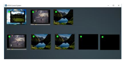
To switch a video source on a display, tap a source object and then tap a display object. The switch takes effect immediately. Alternatively, you can drag-and-drop a source object onto a display object if you have this control action enabled.
