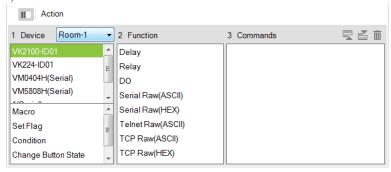
b) Under **Function**, double-click a command to add it to the **Commands** list. This **Command** initiates when the **Condition** is met. For details on Functions and Commands, see *Device Functions*, page 172 and *Advanced Functions*, page 175.
