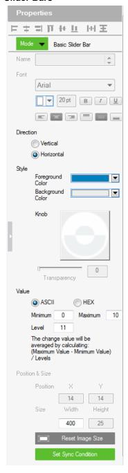
Right click on a Viewer page and select **Slider Bar** to add a bar. A Slider Bar can control a device, link to another page, or run a macro
