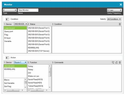
These options are only for advanced setups that require multiple events from hardware devices connected to multiple conditions. Most devices only require one signal Status added to the *Condition List* to initiate an *Action*. Most installations will not need to use this option, therefore it can be ignored.
