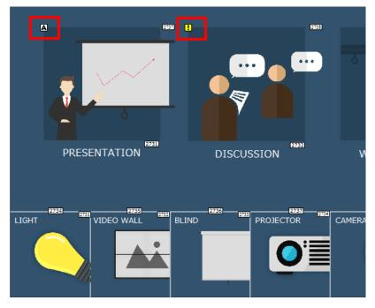
Each object is identified by an ID at the top right corner. These IDs are assigned in the order of creation. These IDs help identify a label when configuring a **Change Label** (page 184) or a button when configuring a **Change Button State** (page 183).
