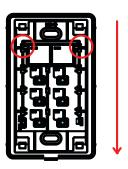
**Caution:** When removing button caps, place your fingers on the top of button caps and then press downwards, as illustrated below. Pressing upwards from the bottom may cause damages to the button caps.
