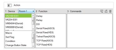
6. Under **Function**, double-click a command to add it to the **Commands** list. This is the **Command** that initiates when the **Condition** is met. For details on what each function does, see *Device Functions*, page 172 and *Advanced Functions*, page 175.
