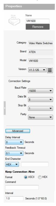
Click a serial device from the Device Configuration list to configure its properties.
