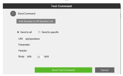
Select which device to send command to by choosing **Send to all** or **Send to specific** and then click **Send Test Command**. This window appears.
