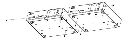
2. Use 4 of the screws from step 2 to secure the two VK1100A / VK1200 units together with the link bracket. Then install the left and right mounting brackets onto the sides of the units using 2 of the M3x5 and M3x6 screws included.
