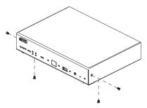
2. Using the 2 bottom screws from step 1 and 2 M3x6 screws from the rack mount kit, secure the mounting brackets to the sides of the VK1100.
