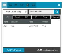
5. Click **Add to Project**. This computer, identified as an Ethernet device installed with ControlAssist, appears in the Device Configuration List.
