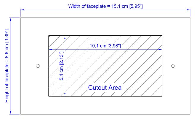
**Note:** ATEN recommends a 2-gang wall box with a depth of at least 5 cm (1.97 inches) to accommodate the connectors and cables.
