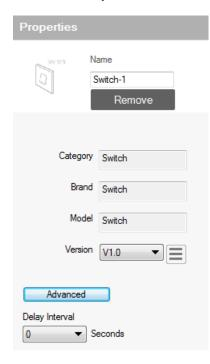
Click an I/O device from the Device Configuration list and select **Input** (VDC), Input (Dry Contact), or Output to configure its properties.
