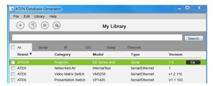
2. Add a command by clicking + and double-click the command column to type the command of requesting for the cumulative lamp usage (hour). Consult the user manual for the device to find out the operation command.
