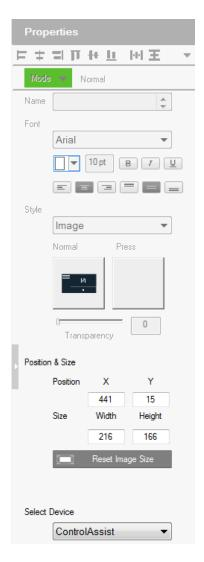
Click a PowerPoint control template or a media control template to configure its position, size, and the PC that controls it.
