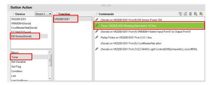
c) To configure the timer, double-click the added timer in the Commands column and select from the drop-down menus.
