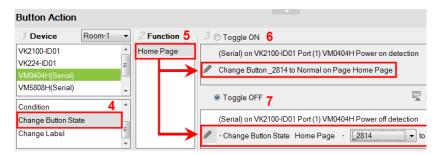
8. In each Commands list, double-click the **Change Button State** command to set the **Button** and **State** (*Normal* or *Pressed*).
