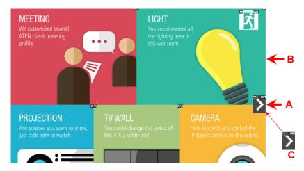
When the top button (A) is pressed, the lowest button (C) is executed.
