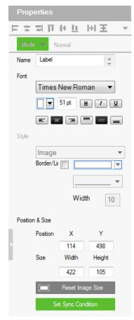
The *Label* properties provide settings for the displayed text and its format.
