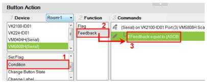
4. Double-click **If Feedback equals to** in the Commands list and use the drop-down menu to select **equal to** or **include** and enter the **Text**.
