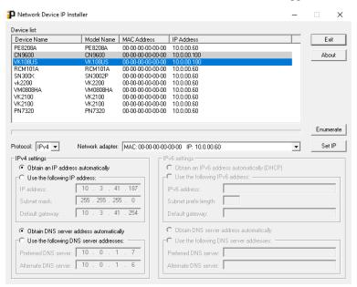
Make sure the proper network adapter is selected and click **Enumerate** to search for and display your ATEN controllers within the *Device List*.
