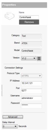
Click an Ethernet device to configure its properties.
