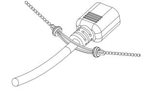
Plug the power cord into the PDU's power outlet, and thread one end of the Lok-u-Plug Cable Holder into the lower left hole next to the power outlet.
