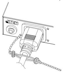
Using a Lok-u-Plug Installation Tool, lock the part of the Cable Holder inserted into the hole by pushing it towards the small part of the hole.
