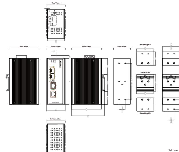
Figure 2: IGUP-2205AT Three-View Diagram
