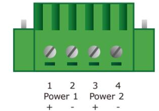
**Note** The wire gauge for the terminal block should be in the range between 12 and 24 AWG.
