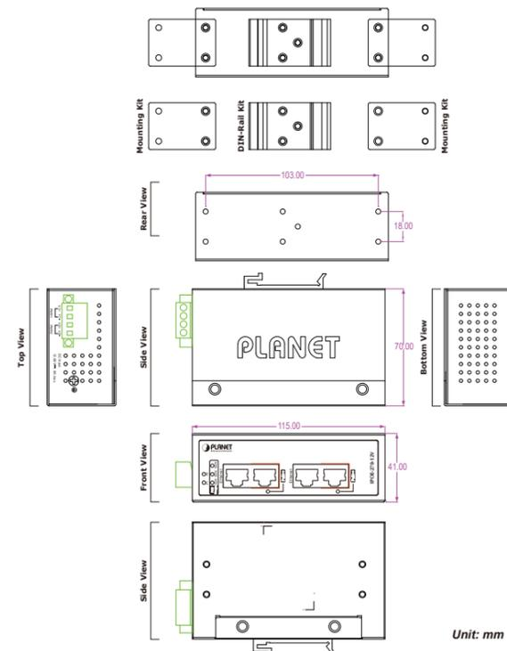
Figure 6: IPOE-270-12V Three-View Diagram
