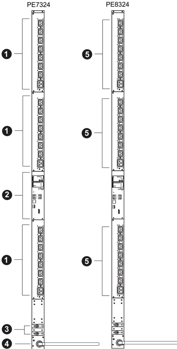
**Note:** The PE7324 / PE8324 unit components are identical except for the outlet LEDs — the PE7324 has none while the PE8324 has 24, as shown by number 5 above.
