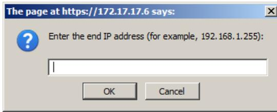
3. To filter a single IP address, key in the same address as the start IP. To filter a continuous range of addresses, key in the end number of the range (for example, 192.168.0.225).
