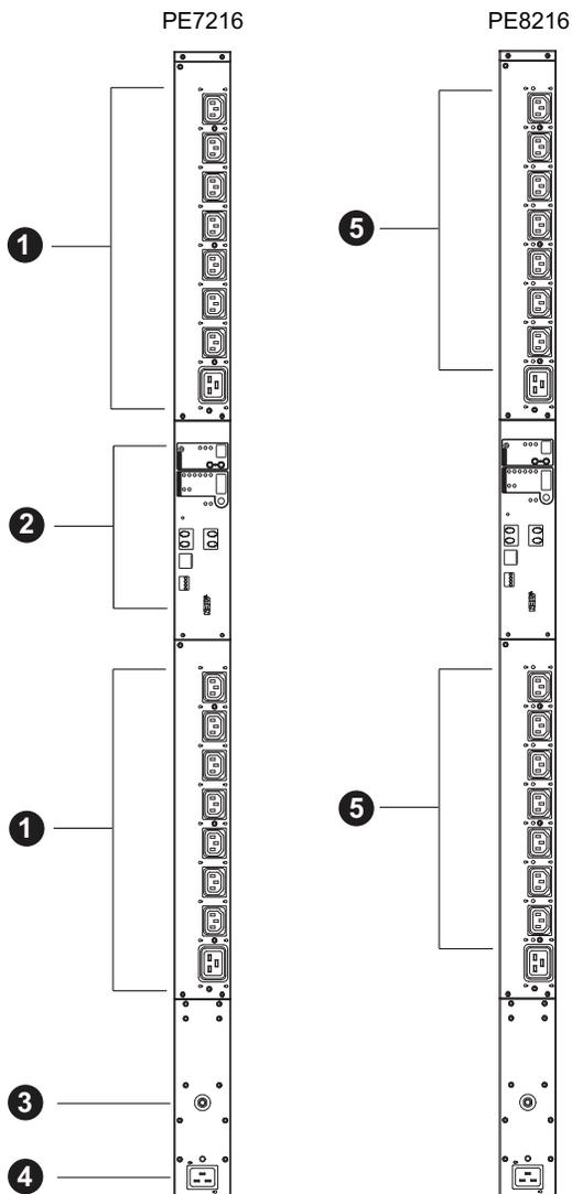
**Note:** The PE7216 / PE8216 unit components are identical except for the outlet LEDs—the PE7216 has none while the PE8216 has 16, as shown by number 5 above.
