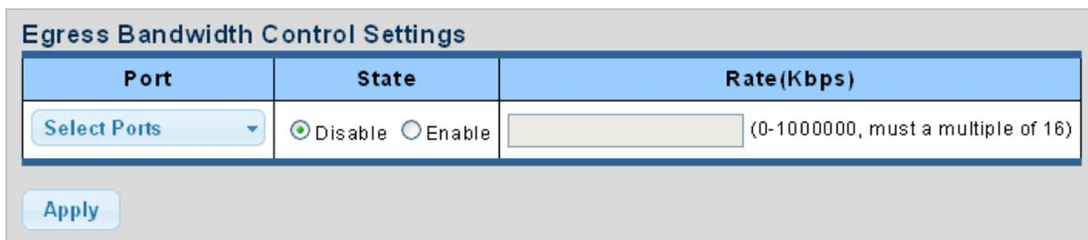
The screenshot shows a configuration page titled "Egress Bandwidth Control Settings". It features a table with three columns: "Port", "State", and "Rate (Kbps)". The "Port" column contains a dropdown menu labeled "Select Ports". The "State" column has radio buttons for "Disable" (selected) and "Enable". The "Rate (Kbps)" column has a text input field with a placeholder "(0-1000000, must a multiple of 16)". Below the table is an "Apply" button.
