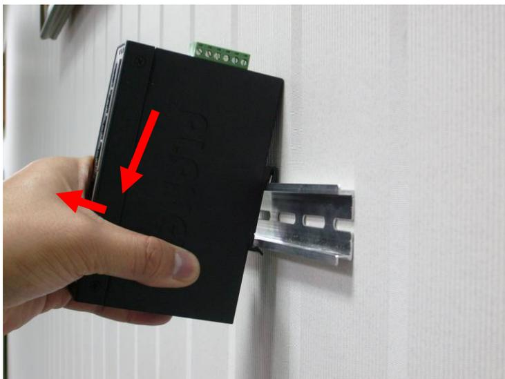
**Step 5:** Lightly pull out the bottom of DIN-rail to remove it from the track.
