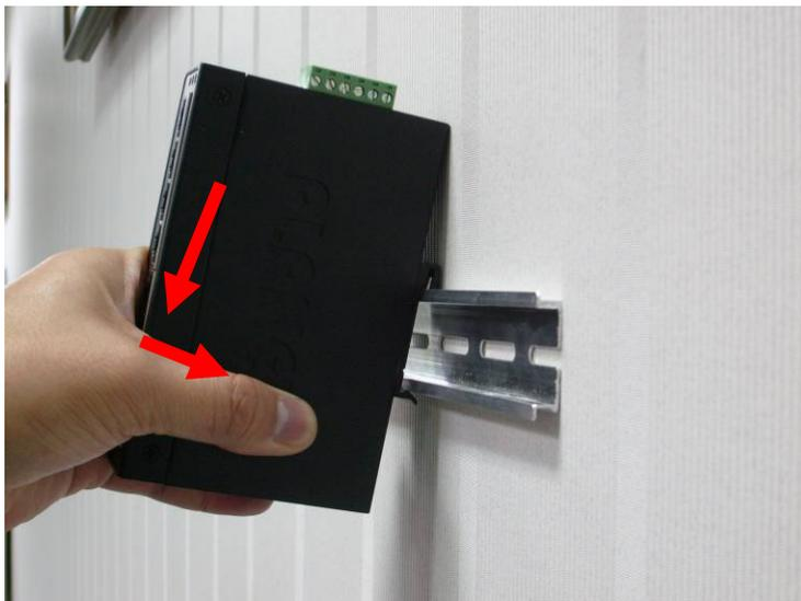
**Step 2:** Place the bottom of DIN-rail lightly into the track.
