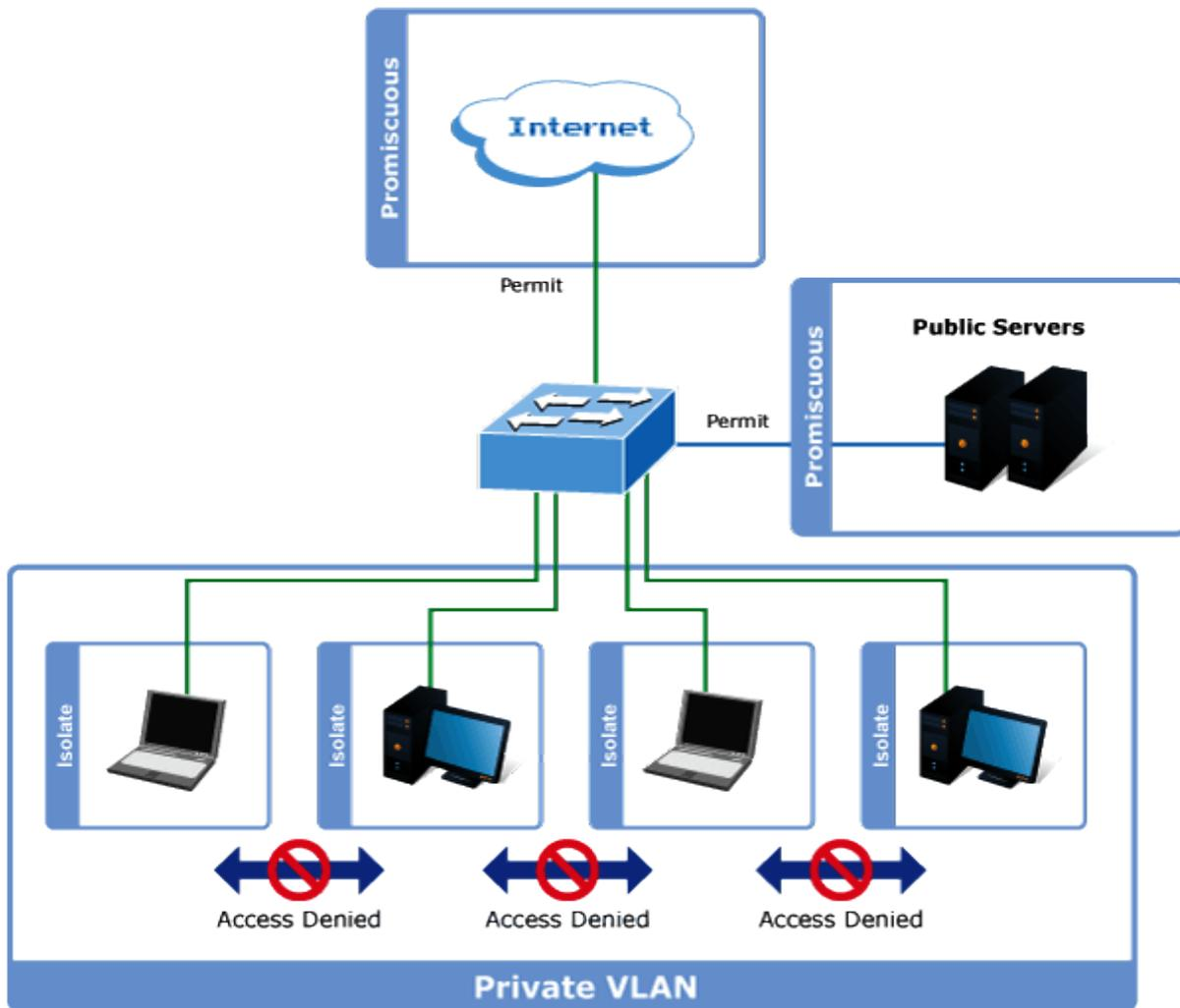
For protected port group to be applied, the Industrial Managed switch must first be configured for standard VLAN operation.
