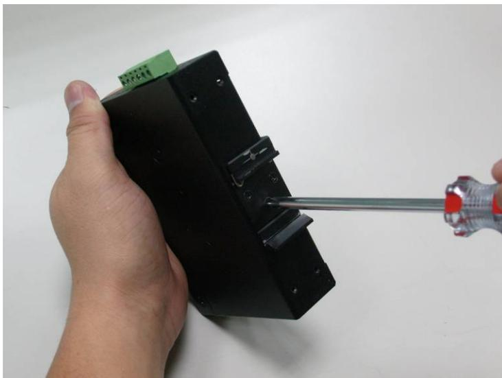
**Step 1:** Screw the DIN-rail on the Industrial Managed Switch.
