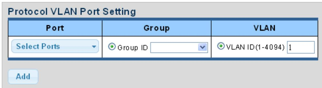
The screenshot shows a form titled "Protocol VLAN Port Setting". It contains three main input fields: "Port" with a "Select Ports" dropdown menu, "Group" with a "Group ID" dropdown menu, and "VLAN" with a "VLAN ID(1-4094)" text input field containing the value "1". Below these fields is an "Add" button.
