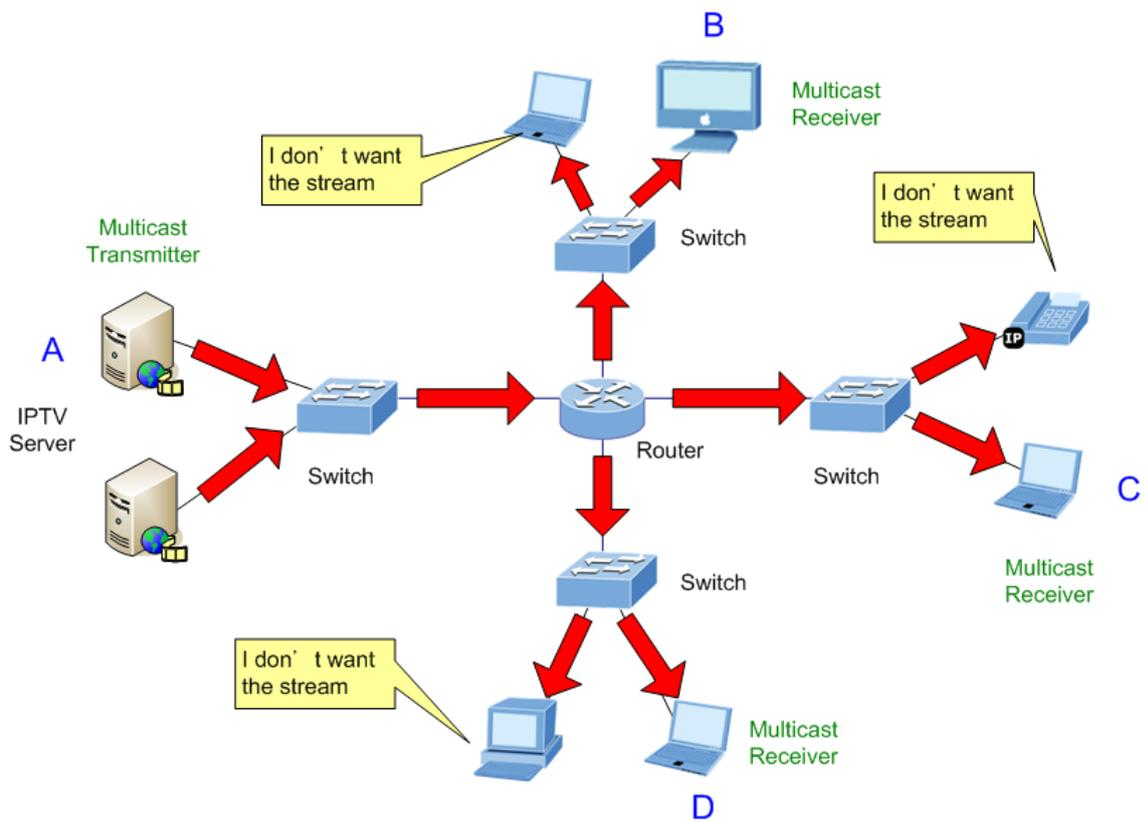
Figure 4-7-4 Multicast Flooding
