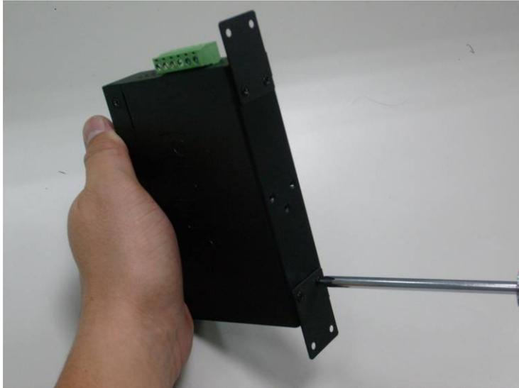
**Step 3:** Use the screws to screw the wall mount plate on the Industrial Managed Switch.
