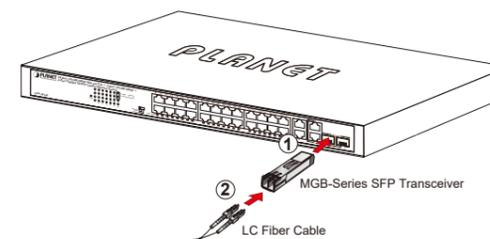
Figure 5-3: Plugging In the SFP Transceiver
