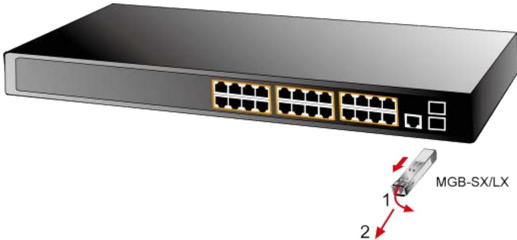
**Figure 2-1-33:** How to Pull Out the SFP Transceiver
