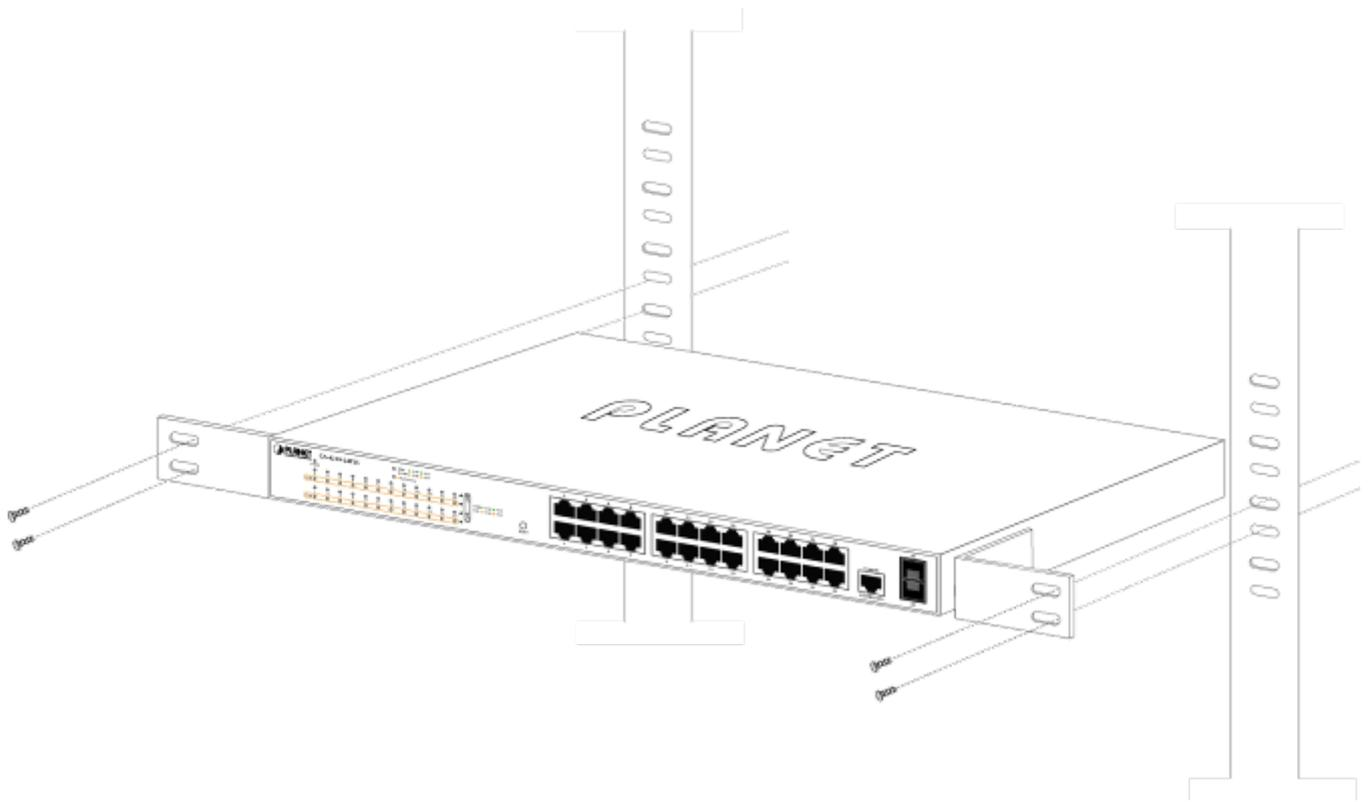
**Figure 2-1-31:** Mounting Managed Switch in a Rack
