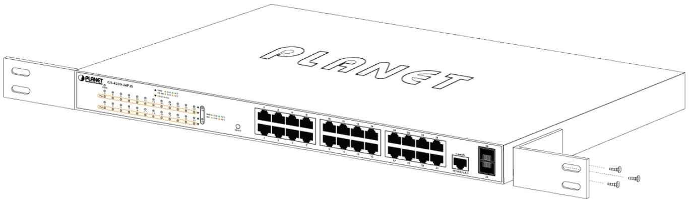
**Figure 2-1-30:** Attach Brackets to the Managed Switch
