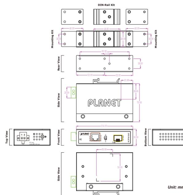
Figure 1: IGTP-815AT Three-View Diagram
