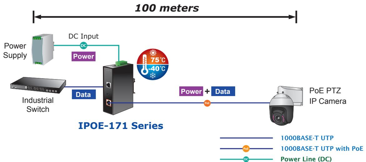
*Installation of 802.3bt PoE Injector and Splitter*
