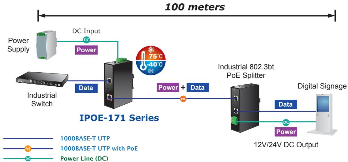
*Extended Installation of IEEE 802.3bt Injector and PoE Network*
