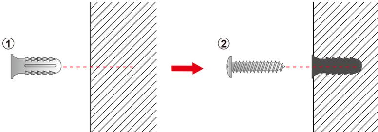
**Step 2:** Place two anchors inside the hole by hammering them. Then screw the two screws leaving a space of 2mm apart as shown in the circled diagram below.
