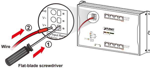
**Step 3:** Remove the flat-blade screwdriver from the release hole.
