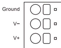
Insert positive/negative DC power wires into Contacts V+ and V- for Power.
