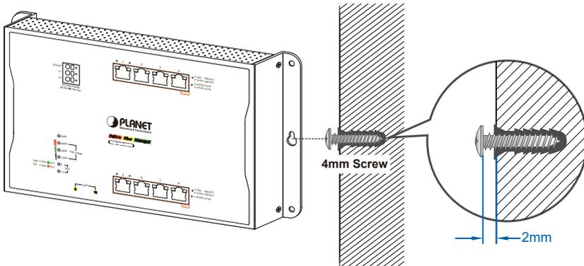
**Step 3:** The switch, shown in the picture below, can now be hung on the wall.
