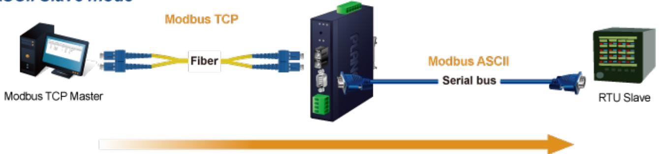
Figure 4-5-9: ASCII Slave Mode Topology
