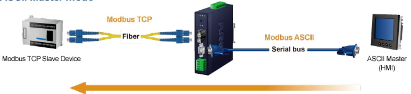
Figure 4-5-11: ASCII Master Mode Topology
