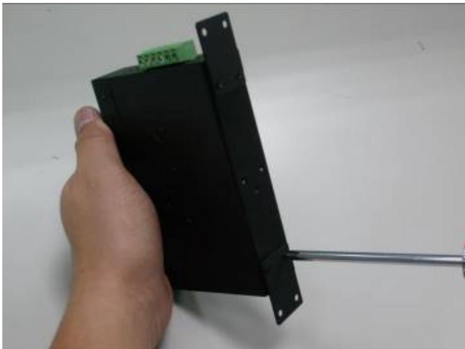
**Step 3:** Use the screwdriver to screw the wall-mount plate on the **Modbus Gateway**.
