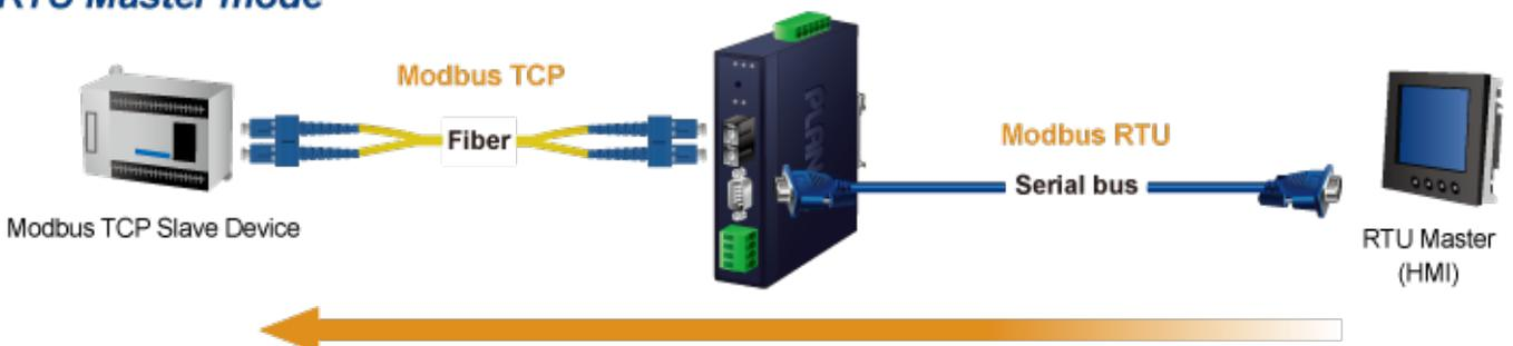
Figure 4-5-7: RTU Master Mode Topology
