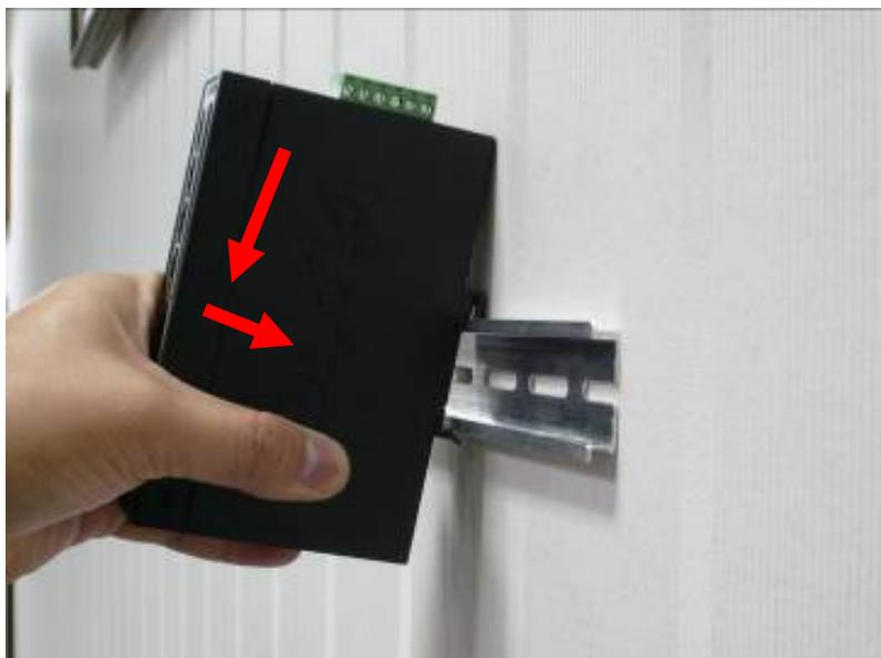
**Step 3:** Check whether the DIN-rail bracket is tightly on the track.
