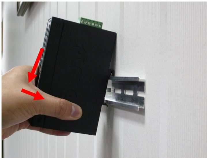
**Step 2:** Place the bottom of DIN-rail bracket lightly into the track.
