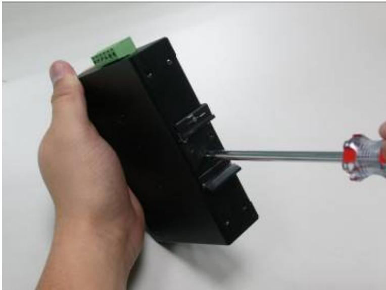
**Step 2:** Lightly place the upper bracket into the DIN rail and push the unit down till the lower bracket is locked into the track.
