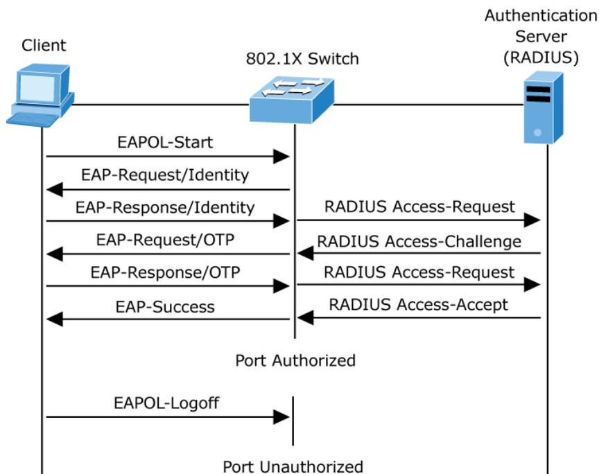
Figure 4-5-2-2: EAP Message Exchange
