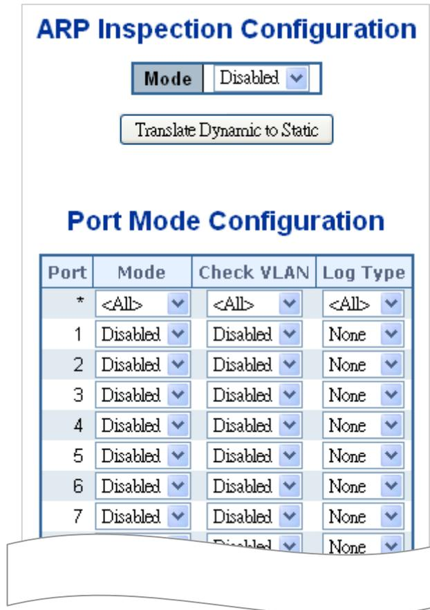
Figure 4-5-8-1: ARP Inspection Configuration Screen Page Screenshot
