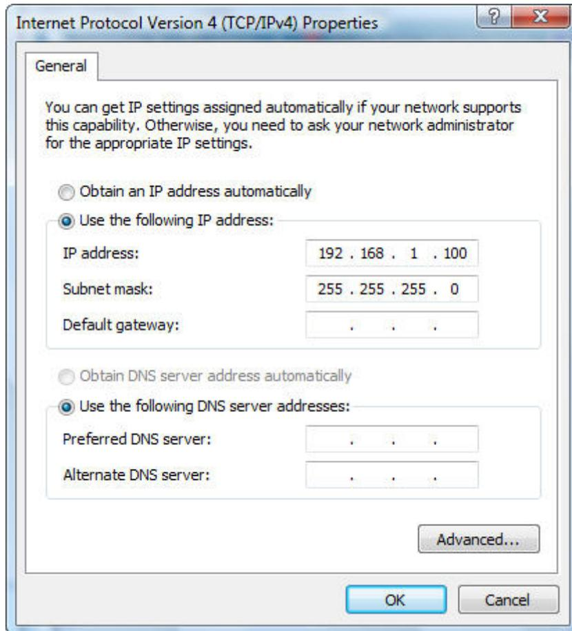
**Figure 4-1** TCP/IP Setting
