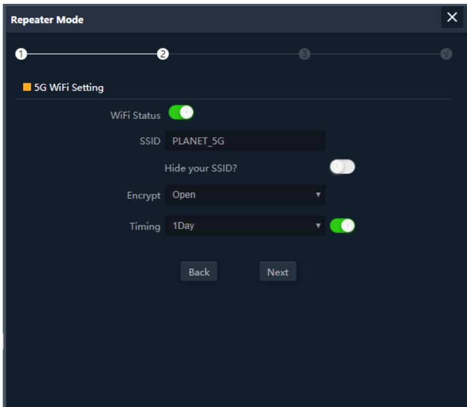
Figure 5-18 Repeater Mode – Setting up Wi-Fi
