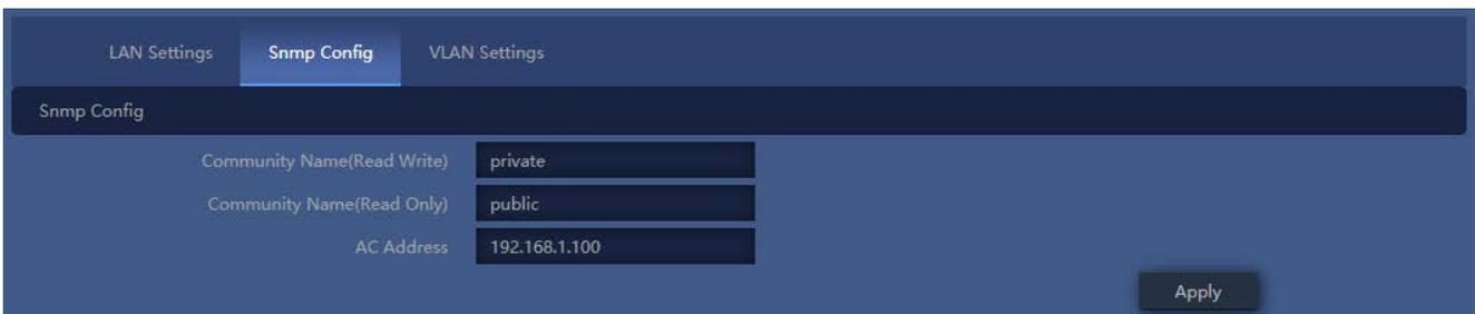
Figure 5-10 SNMP Config
