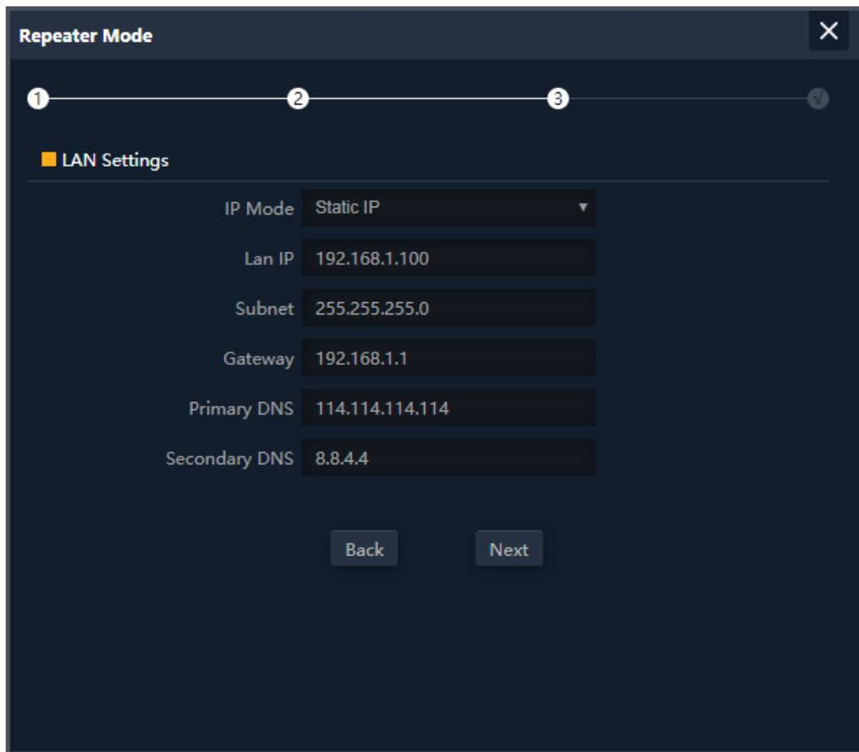
Figure 5-19 Repeater Mode – Setting up Wi-Fi
