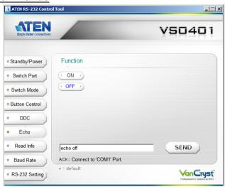
The Echo function, when enabled, lets the VS0201 / VS0401 perform operations received via the front panel pushbuttons, web GUI and and IR controller, but not corresponding commands received through the RS-232 interface.
