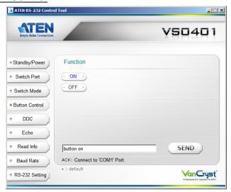
Button Control function allows you to secure your device by locking the use of front panel pushbuttons.
