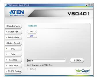
The DDC function, when enabled, lets the VS0201 / VS0401 check the connected display to provide correct updated EDID information to the source device so that the display is optimized accordingly. With Dynamic DDC off, the source devices do not receive updated EDID data, which can cause display issues. If there is a problem with your display quality, however, it is recommended that Dynamic DDC be turned off.
