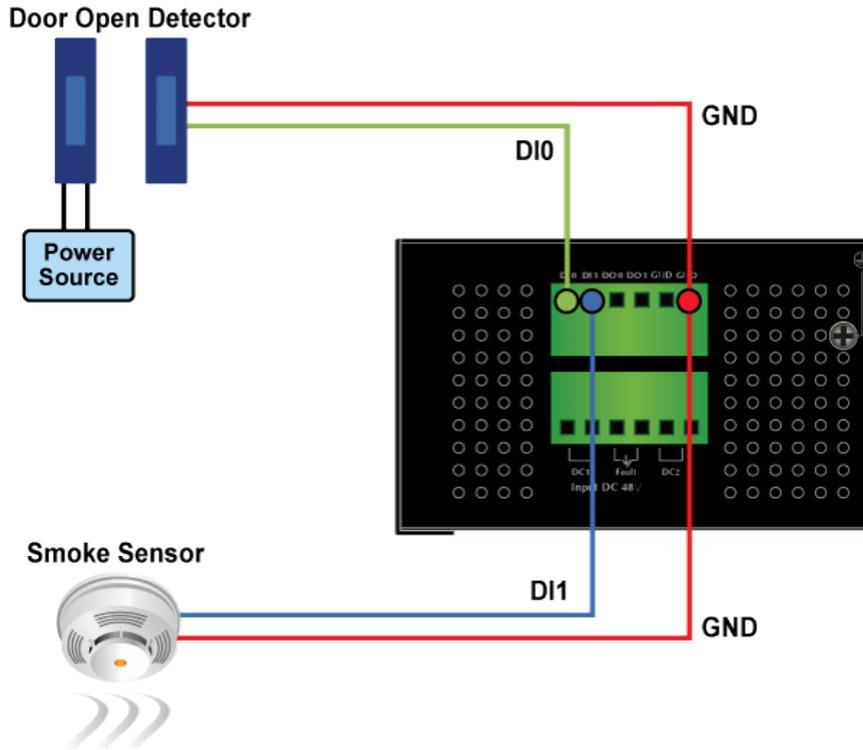
Figure 2-1-15 Wires D10 and D11 to Open Detector
