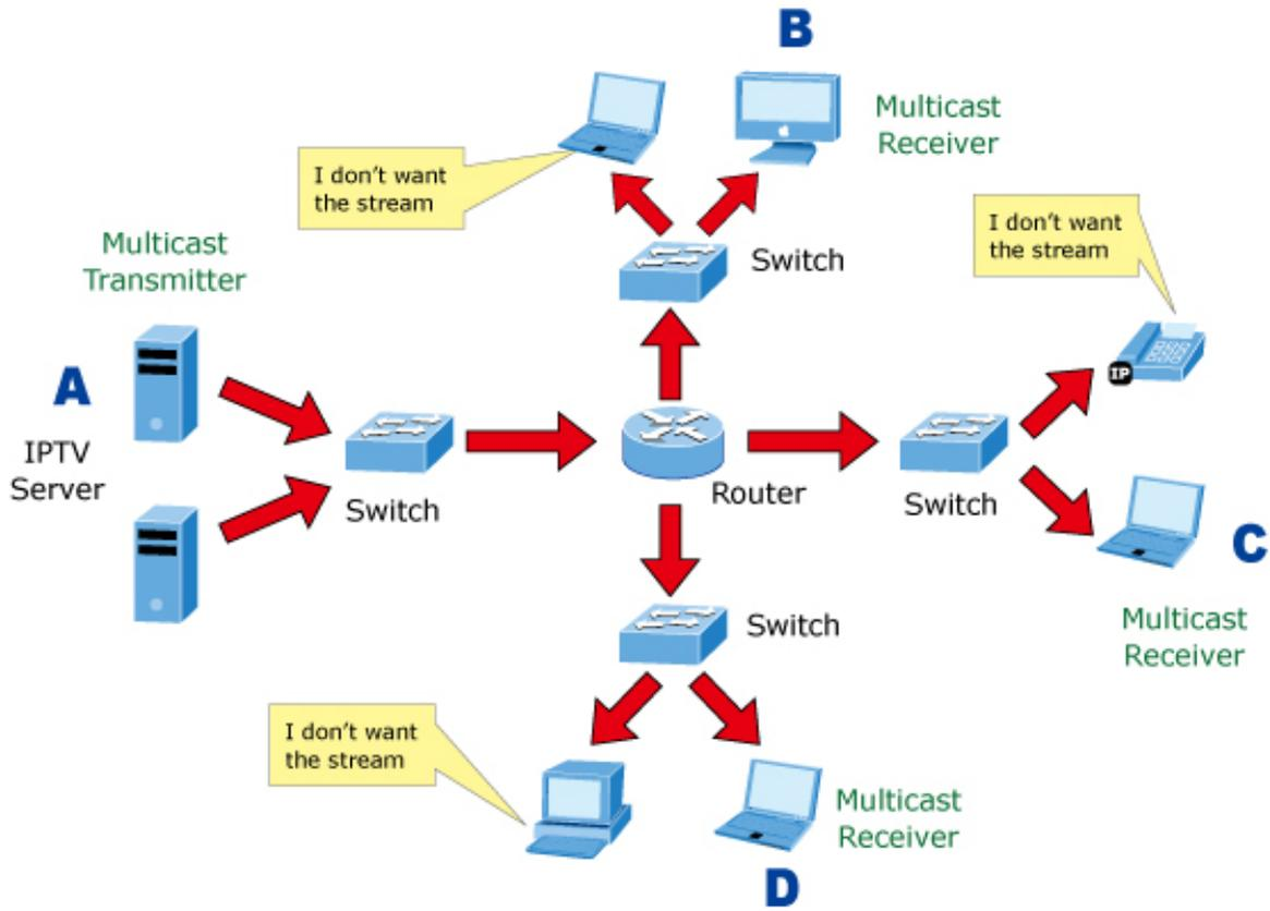
Figure 4-3-5-2: Multicast Flooding
