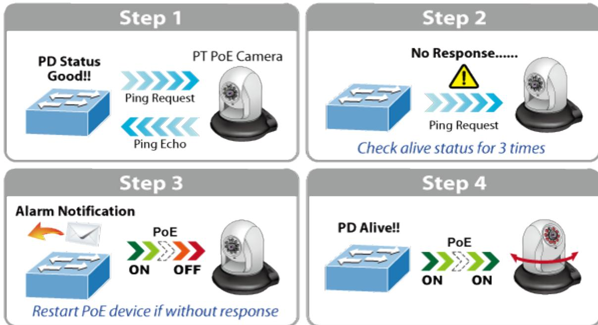
This page provides you how to configure PD Alive Check. The screen in Figure 4-8-1-7 appears.
