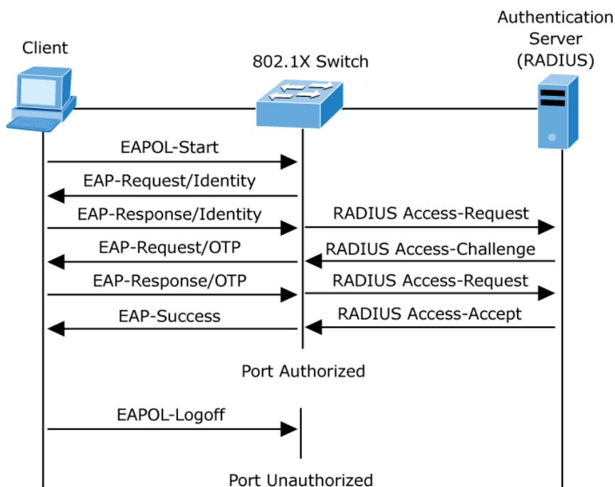
Figure 4-5-2-2: EAP Message Exchange
