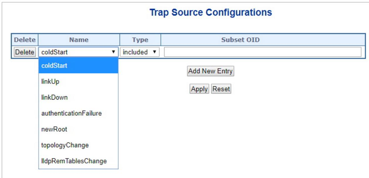
Figure 4-2-2-6: SNMP Trap Source Configuration Page Screenshot
