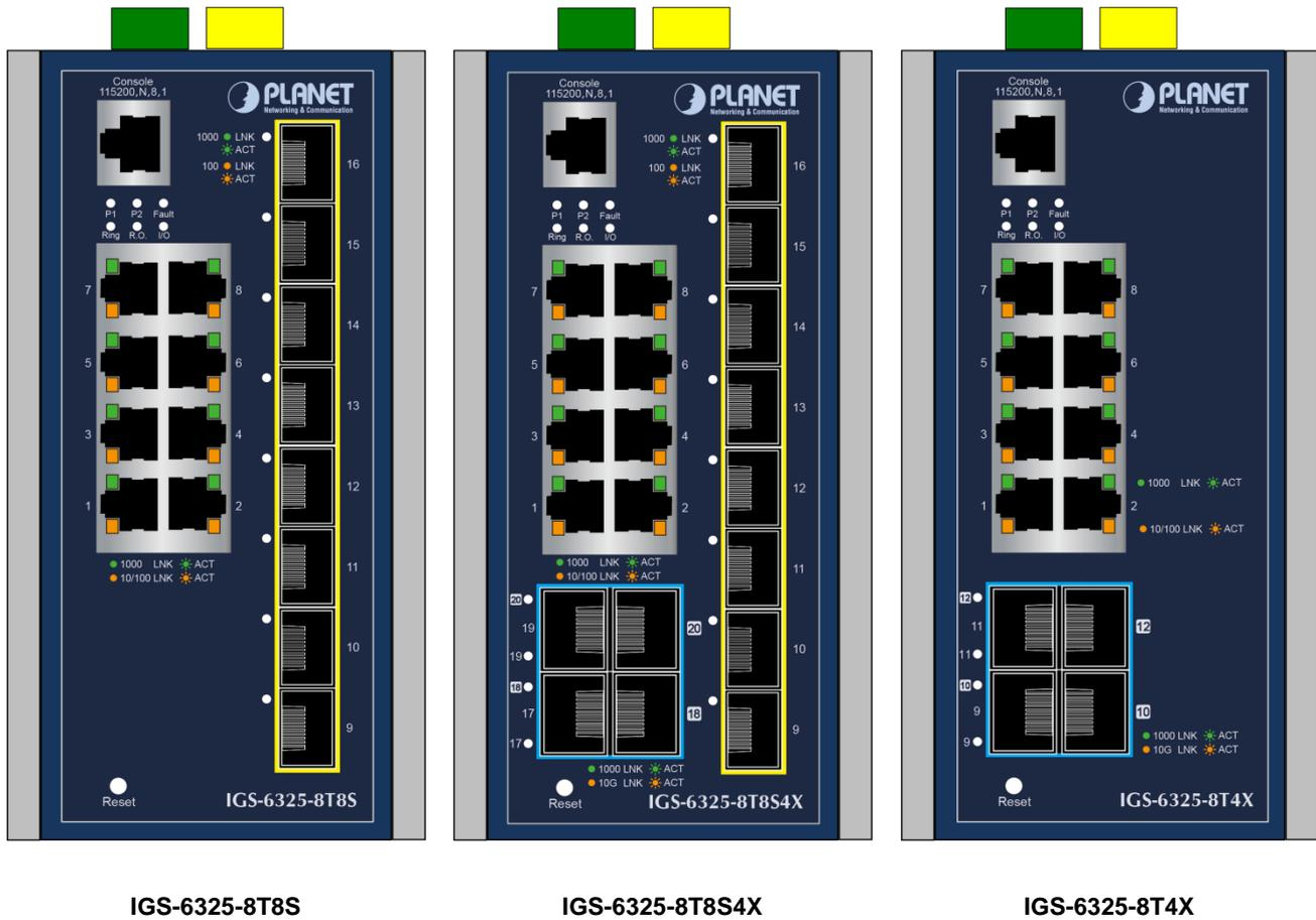
Figure 2-1-3 IGS-6325-8T8S and IGS-6325-8T8S4X Switch Front Panels
