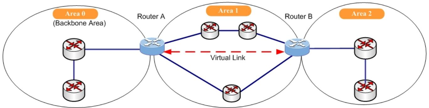
Following is OSPF virtual link configuration table. The virtual link is established between 2 ABRs to overcome that all the areas have to be connected directly to the backbone area. The screen in [Figure 4-10-4-8](#) appears.
