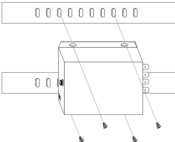
**Wall Mount:** Mount device on the wall with screws
