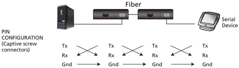
From a source device, the RS-232 signals is transmitted (Tx) to the VE883 receiving (Rx) unit; the VE883R transmits (Tx) signals to the display device (Rx).
