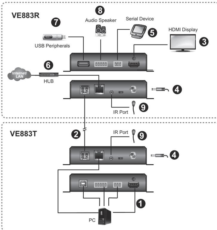
1. Connect your source device to the VE883T. To transmit HDMI video/stereo audio/USB/serial/Ethernet signals, connect the source device's HDMI Out/Audio Out/USB/RS-232 Serial/Ethernet port to the VE883T.
